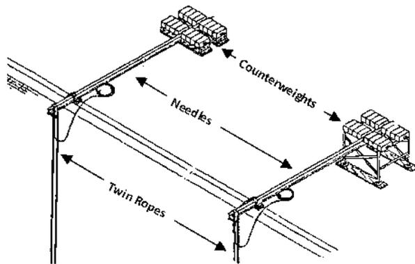
Figure 15b. Suspended (swing-stage) scaffold – Cradle (suspended) end
