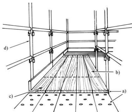
**Figure 4.** Overlapping planks. Lapped scaffold planks may sometimes be used to cover gaps around corners of scaffold bays. These planks generally may not need to be secured, provided the following are met:
