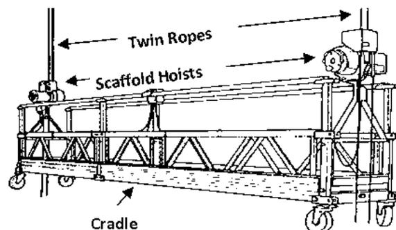
The following control measures should be implemented for a suspended scaffold:
