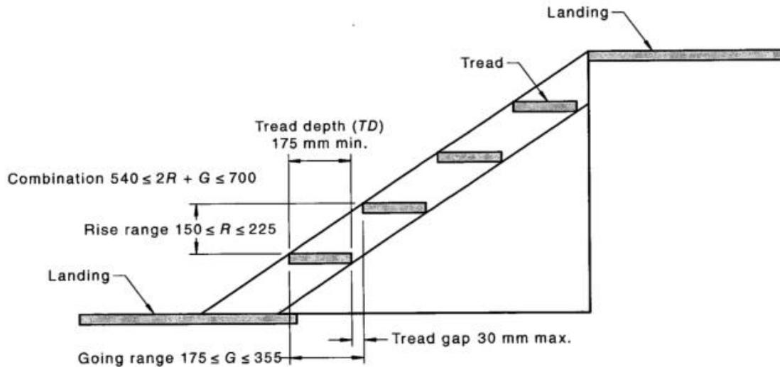
**Figure 5.** Temporary stairway configuration
