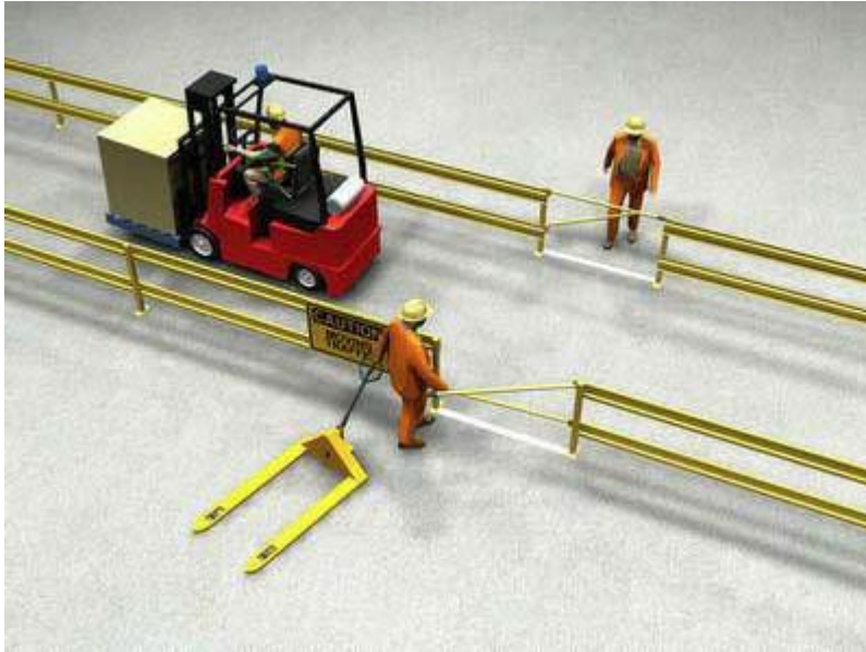
Barrier system in combination with pedestrian gates
