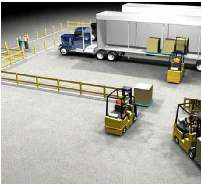
Loading/receiving area with truck drivers physically separated from forklifts
