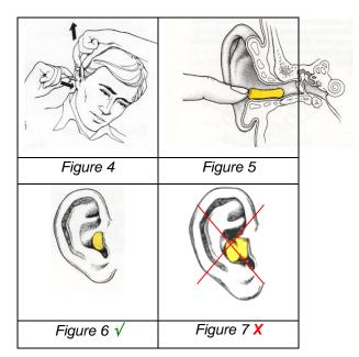
With the earplug inserted in the ear canal it should sit as shown in Figure 6, and when looking front-on should be hidden (most of it at least) behind the lump (tragus) at the front of the outer ear. If the earplug is inserted as in Figure 7 it is not deep enough in the ear canal and does not provide the protection needed for it to do its job.
