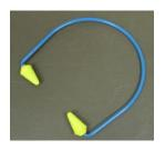
Semi-insert plugs (as illustrated) and ear canal caps seal the ear canal at or near its entrance. They are held in position by a tension band which is normally worn under the chin or behind the neck.
