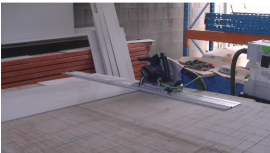
Figure 4: On-tool extraction using backer-board.
