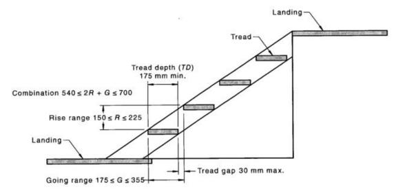
Figure 5. Temporary stairway configuration
