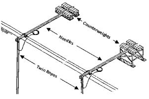
**Figure 15b.** Suspended (swing-stage) scaffold – Cradle (suspended) end
