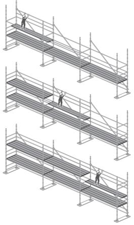
Figure 10 Scaffold erection<sup>2</sup>
