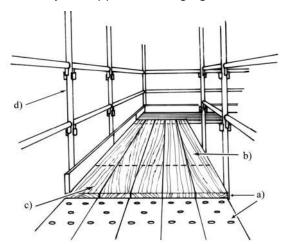
**Figure 4.** Overlapping planks. Lapped scaffold planks may sometimes be used to cover gaps around corners of scaffold bays. These planks generally may not need to be secured, provided the following are met:
