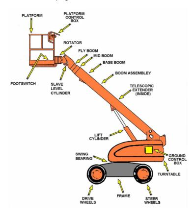
Figure 2.2: Typical EWP with telescoping knuckle boom
