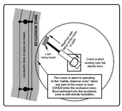
The safety observer zone is designed to encourage plant operators to locate their equipment so that the risk of it entering the exclusion zone is minimal. When this is not possible, adopt other suitable precautions to prevent encroachment into the exclusion zone.
