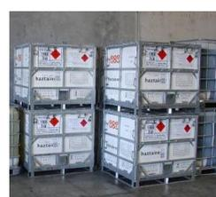
**Figure 1:** Static tanks and transportable containers such as isotainers and intermediate bulk containers (IBCs) are examples of bulk containers (i.e. tanks) requiring a tank placard for Schedule 11 hazardous chemicals at a workplace.
