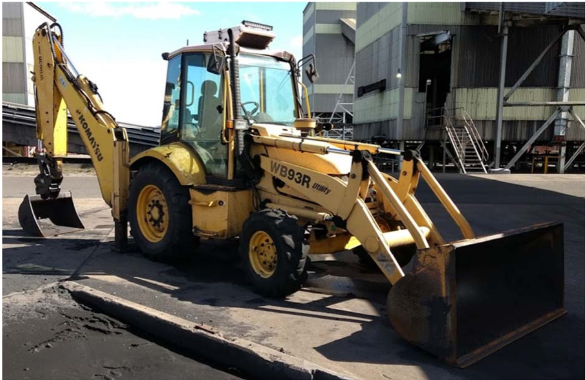
Image 2. Coal plant backhoe with pressurised cabin.
