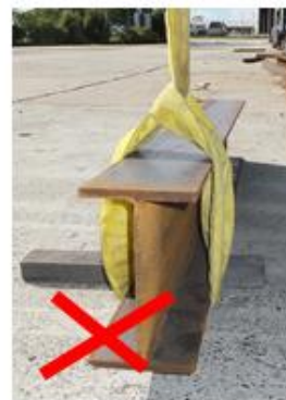
Figure 8: Unsafe use! Edges of I-Beam may cut sling
