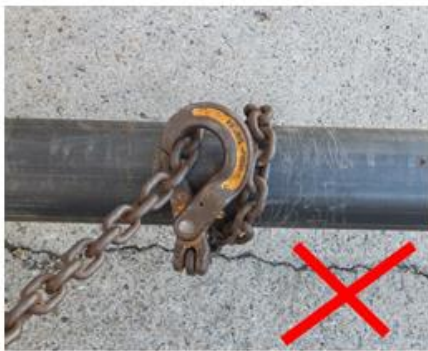
Figure 10: Chain sling with chain bearing against latch
