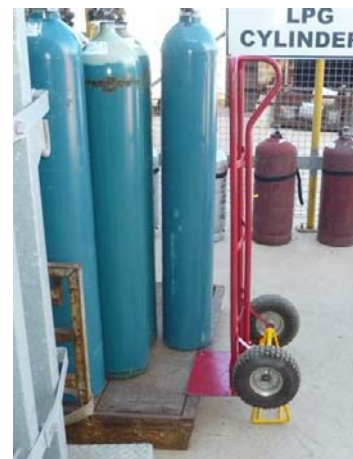
Modified two wheel trolley for improved transfer of plant
