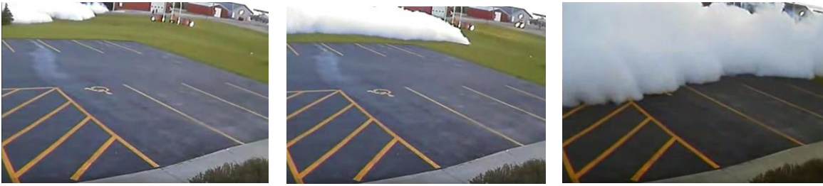
Figure 1: Series of photos showing an ammonia gas cloud travelling from the release point keeping low and travelling along the ground.
