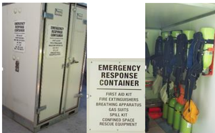
Figure 3: An example of a dedicated ammonia emergency response kit that includes response equipment including SCBA. The unit is portable using a forklift and serves to protect the gear and ensure it is readily available.
