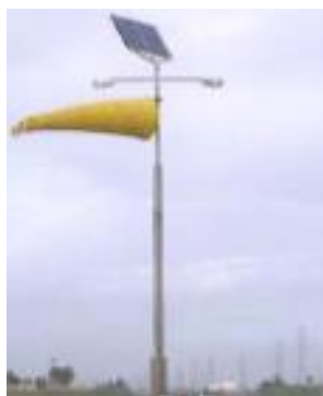
Figure 2: Windsock showing wind direction and likely direction of travel for a vapour cloud.
