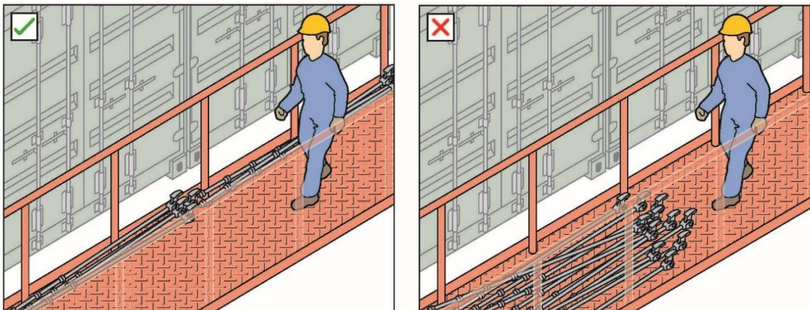
Figure 1 Safe storage of lashing bars to be reused
