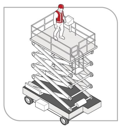
Figure 11 Scissor-lift elevating work platform
