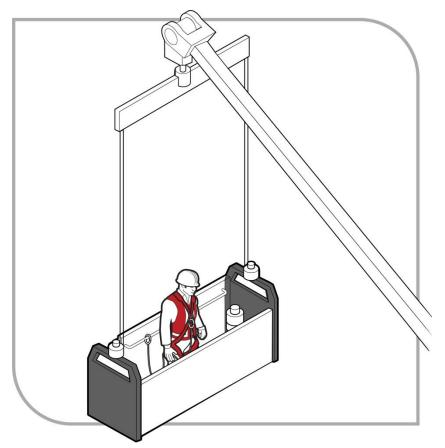
Figure 16 Building maintenance unit with harness and anchor rail
