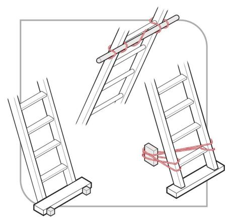
Figure 29 Examples effectively securing a ladder
