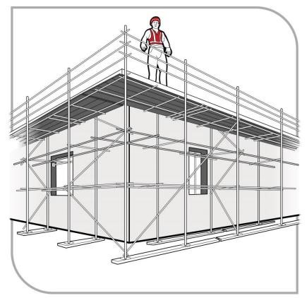
Figure 7 Perimeter scaffold with fully decked working platform, guardrails, mid-rails and toe-boards
