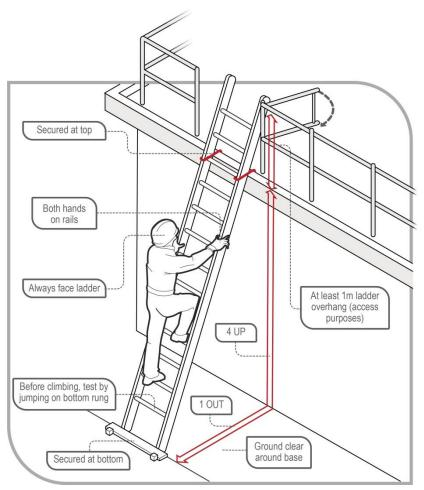
Figure 30 Example of acceptable ladder use
