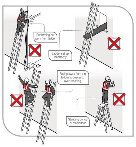
Figure 31 Examples of unsafe ladder use
