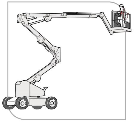
Figure 10 Boom-type elevating work platform
