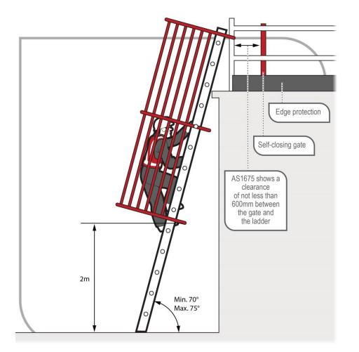
Figure 32 Fixed ladder with ladder cage
