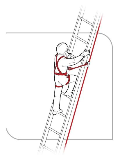
Figure 25 Anchorage line system
