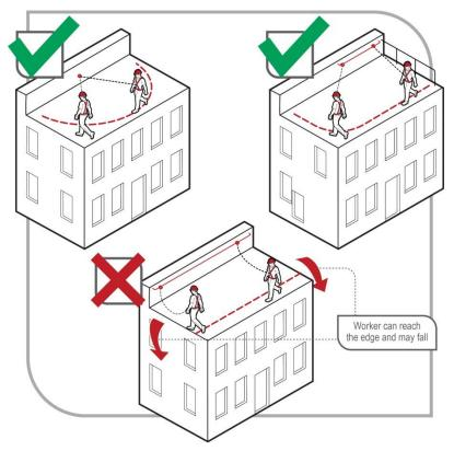
Figure 19 Restraint technique options
