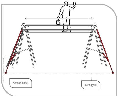
Figure 17 Trestle ladder scaffold with guard rails and outriggers for stability
