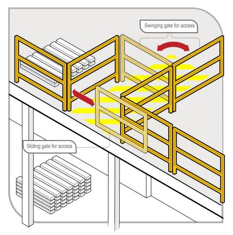
Figure 3 Mezzanine floor barrier
