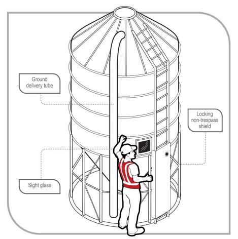
Figure 2 Silo with sight glass and ground delivery tube
