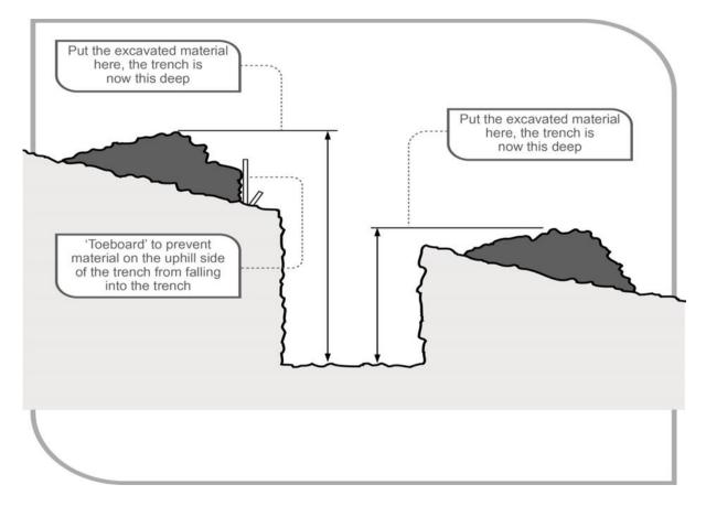
Figure 3 Excavated material impact on effective excavation depth
