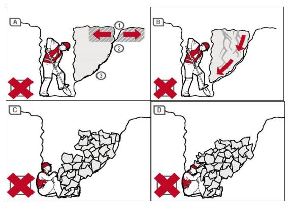
Figure 8 Trench collapse and associated ground forces
