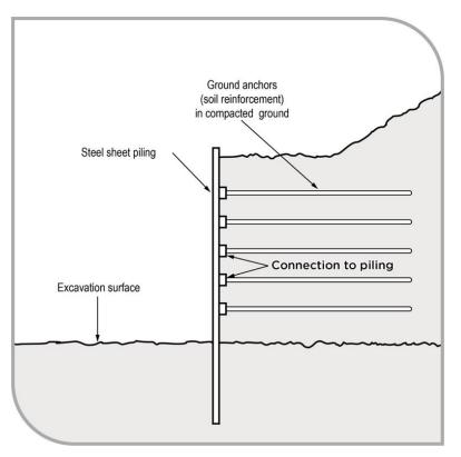
Figure 18 Ground anchors for supporting steel sheet piling
