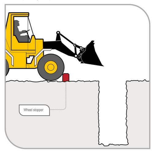
Figure 5 Preventing plant operation near excavations
