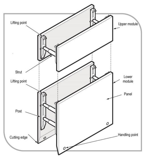
Figure 19 A typical trench shield.
