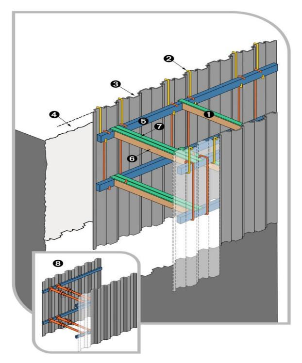
Figure 13 Steel sheet piling
