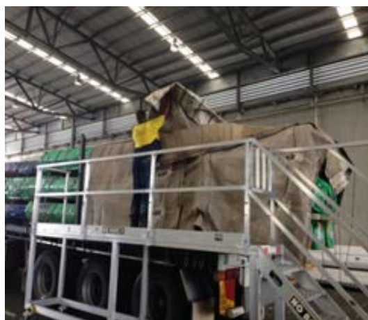
The mobile stand helps prevent workers from having to climb on the trailer
