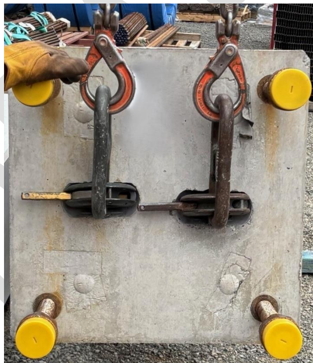
Figure 12 Body (torus) of the lifting clutch perpendicular to direction of rotation
