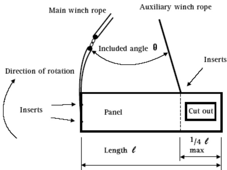
Diagram 12 – Initial position of panel prior to rotation
