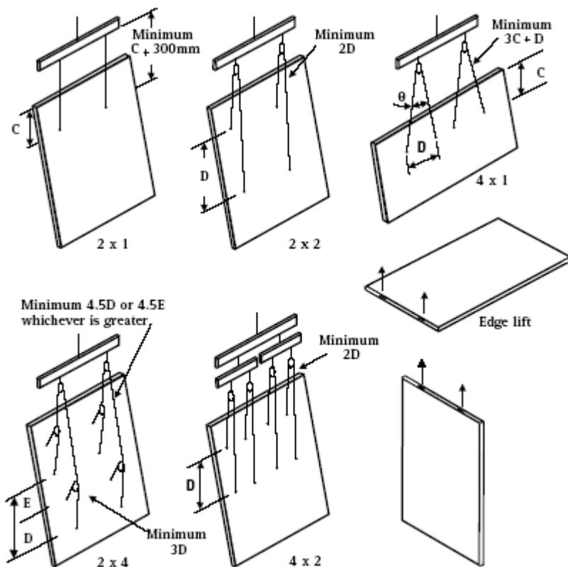
Diagram 10 – Common rigging configurations
