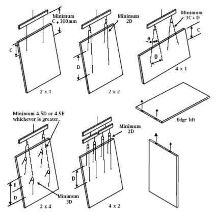
Diagram 10 - Common rigging configurations
