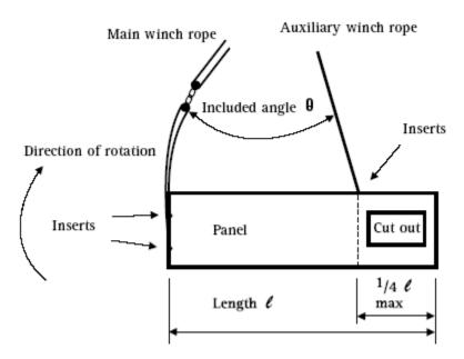
Diagram 12 – Initial position of panel prior to rotation
