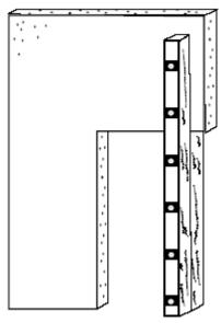
Diagram 5. Unstable panel requiring method of support
