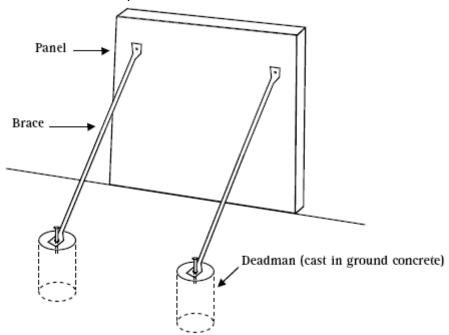
Diagram 4 – Deadman for anchoring braces
