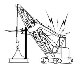
When operating plant near power lines a number of factors must be considered when implementing systems to maintain the "exclusion zone" from overhead power lines. These include the following:
