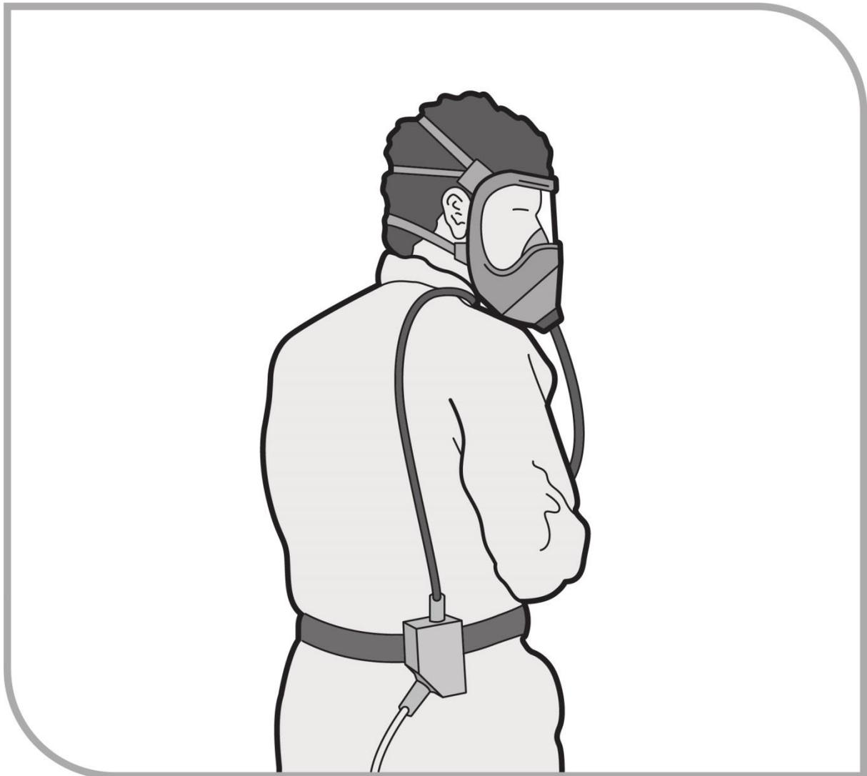
**Figure 14** Full-face, positive pressure demand air-line respirator
