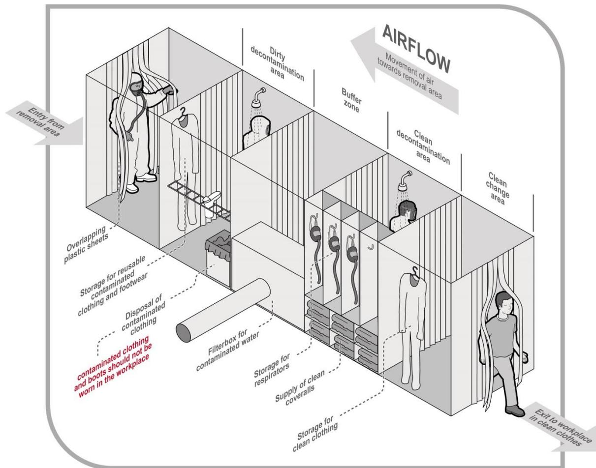
**Figure 4** Decontamination unit
