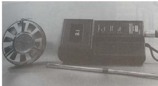
Figure 15: Whirling vane anemometer (l)
