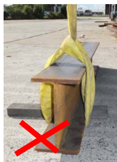
Figure 8: Unsafe use! Edges of I-Beam may cut sling
