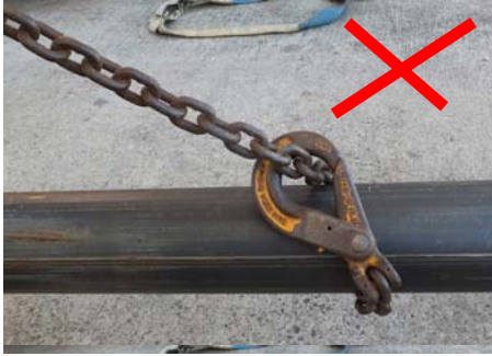
Figure 9: Chain sling with single wrap choke around steel pipe – does not prevent slippage
