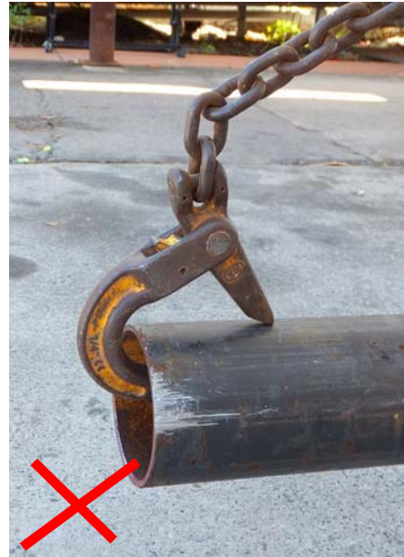
Figure 11: Sling hook inserted into pipe
