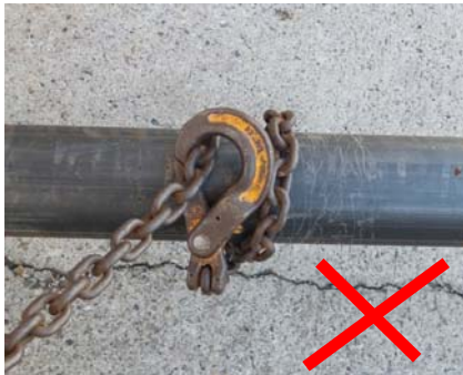
Figure 10: Chain sling with chain bearing against latch
