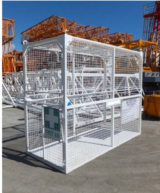
Figure 12 – compliant first aid box
