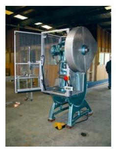
An old style press refurbished with an interlocked safety cage and gate.
