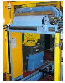
A light curtain used to disable the hazardous mechanism of a machine must resist failure and fault.
