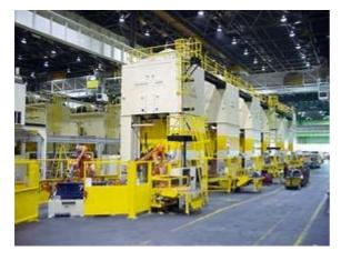
Permanently fixed gantries, ladders and walkways are incorporated into this machinery and equipment to reduce the risk of a fall from height occurring during operation and maintenance.
