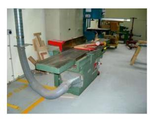
Woodworking dust generated by a buzzer is removed via forced extraction and ventilation.
