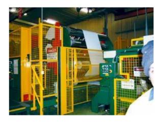
**Tunnel guards** provide a tunnel, aperture or chute in which material can be inserted into the machinery and equipment, but due to the restrictive design and depth of the opening, fingers, hands, arms, or the entire person is prevented from intruding into the danger area.
