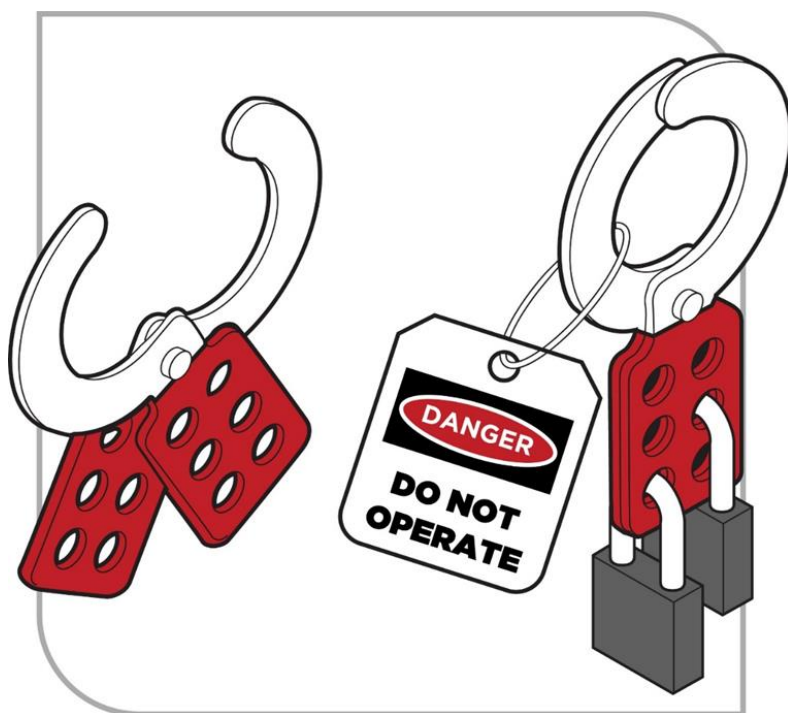
Figure 3 Example of tag and lockout with padlocks
