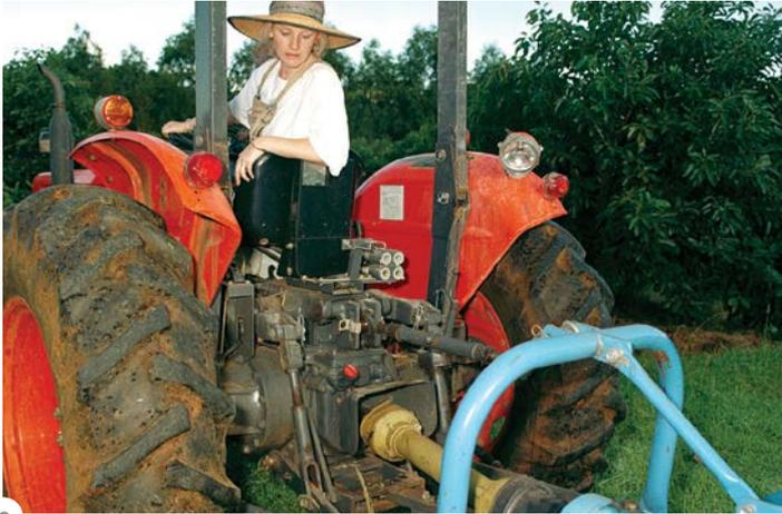
Examples of machinery that need guarding include tractor power take off (PTO) shafts, soil and grain augers, and other belt, chain or sprocket drives. All guarding must comply with the relevant Australian Standards.
