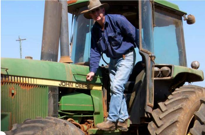
Tractors are used in a variety of farm activities and must include a roll-over protective structure (ROPS) to reduce the risk of injury to the driver in the event of a roll-over.
