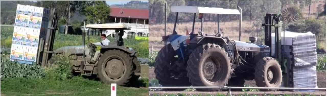
The items of plant pictured below do not fall within the definition of a forklift truck as they do not have a mast and elevating load carriage. Therefore a forklift HRW licence is not required.
