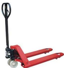
This pallet truck does not fall within the definition of a forklift and a LF licence is not required.
