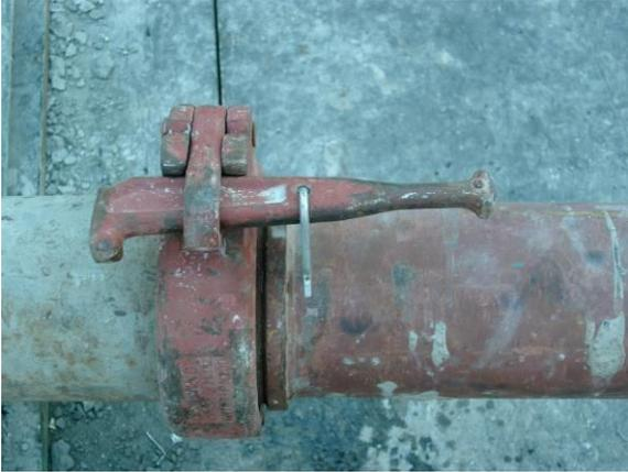
Figure 1. High pressure pipe clamp.
