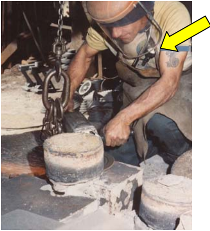
Figure 9: Foundry worker wearing elutriator suitable dust sampler in his breathing zone
