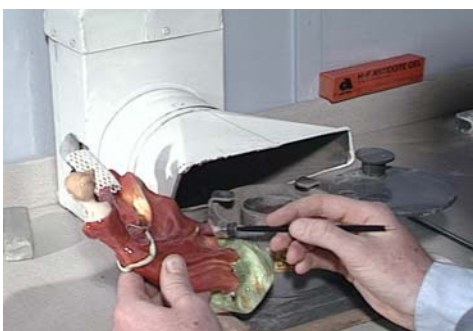
Figure 13A: Fixed exterior hood (HSE UK)
