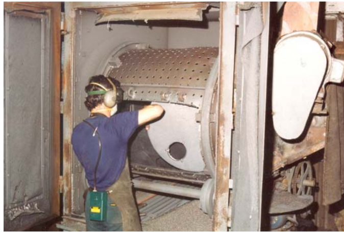
Figure 12: Abrasive blasting with isolating cabinet fitted with LEV
