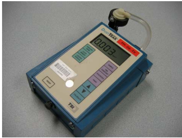
Figure 10: DustTrak™ fitted with cyclone elutriator for static monitoring and checking of dust controls
