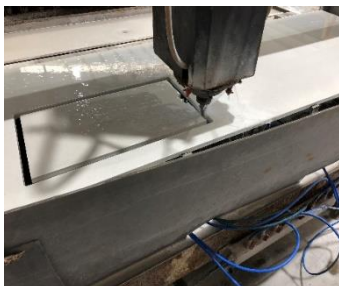
Figure 9 - CNC router without plastic shrouding to contain dust and water mist. Photo by WHSQ.
