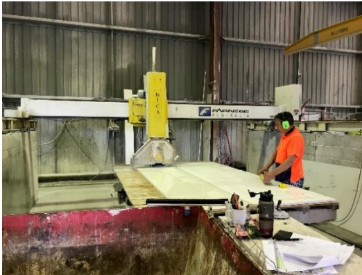
Figure 7- Older manual bridge saws without any means to prevent workers from standing close to the process when operating the saw. Photo by WHSQ.
