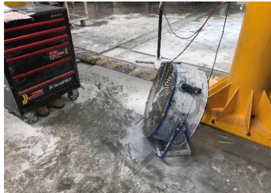
Figure 5 - Photo of dust deposits allowed to dry. Fans may have assisted in drying wet surfaces leaving dry stone deposits.
