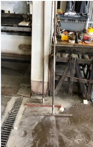
Figure 4 - Instead of dry sweeping, squeegees were commonly used to move stone slurry into floor grates. Photo by WHSQ
