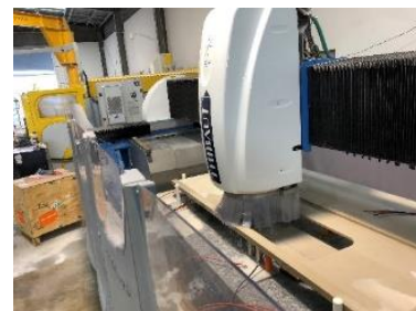
Figure 10 - CNC router with plastic shrouding. Photo by WHSQ.
