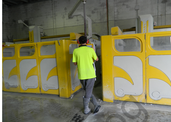
Figure 8 – Newer CNC bridge saws were fitted with bay doors. Photo by WHSQ.
