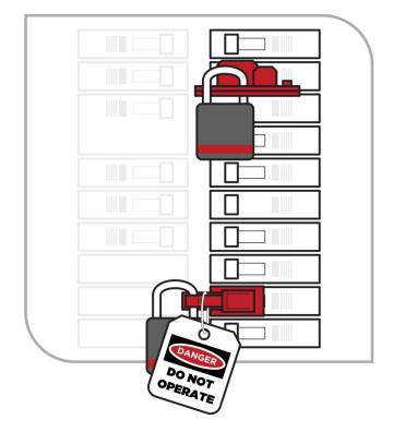
Figure 6 Locking off methods incorporating danger tags—danger tagged circuit breaker locking-off devices
