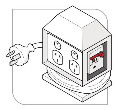
Figure 4: Portable safety switch protected power board
