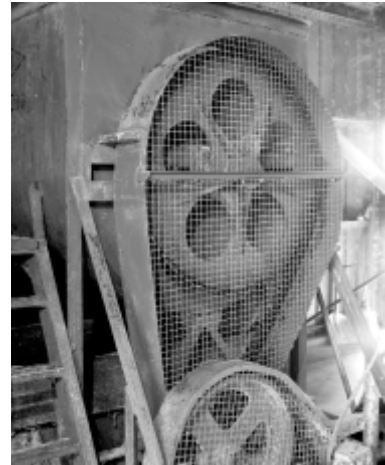
Figure 2. Demonstration of guarding as an appropriate method of separating workers from risk.
