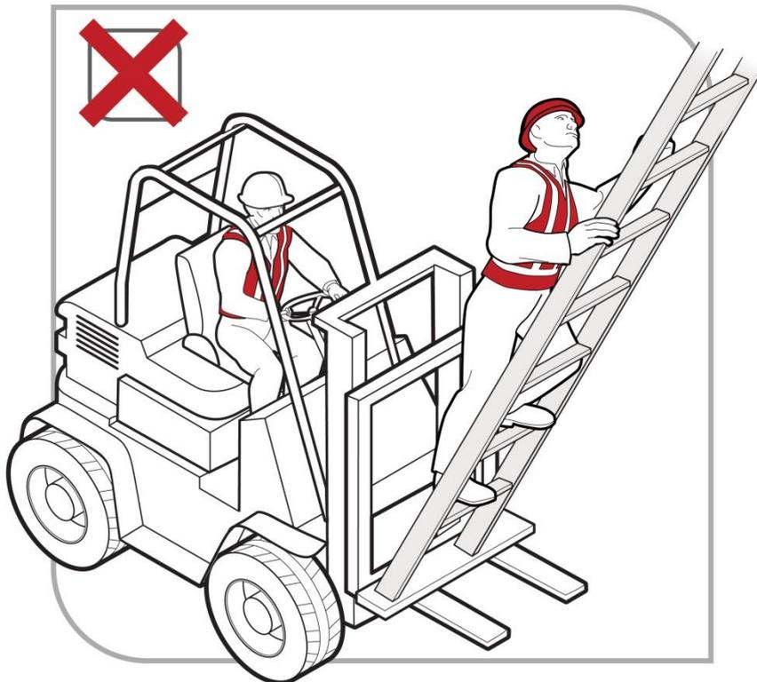
**Figure 15** Unacceptable practice with ladder on forklift
