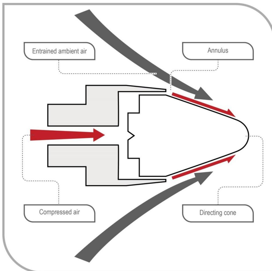
**Figure 7** Example of a pneumatic nozzle (entraining unit)
