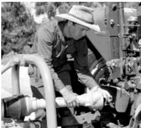
Figure 1. Tractor being fitted with PTO guard.
