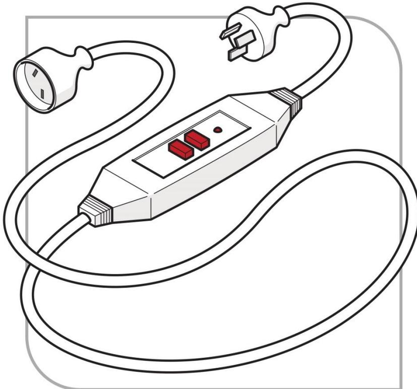
**Figure 3:** Portable RCD fitted directly to power cable
