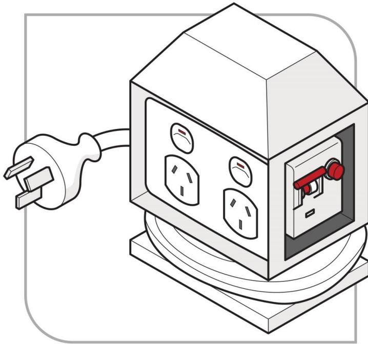
**Figure 4:** Portable safety switch protected power board
